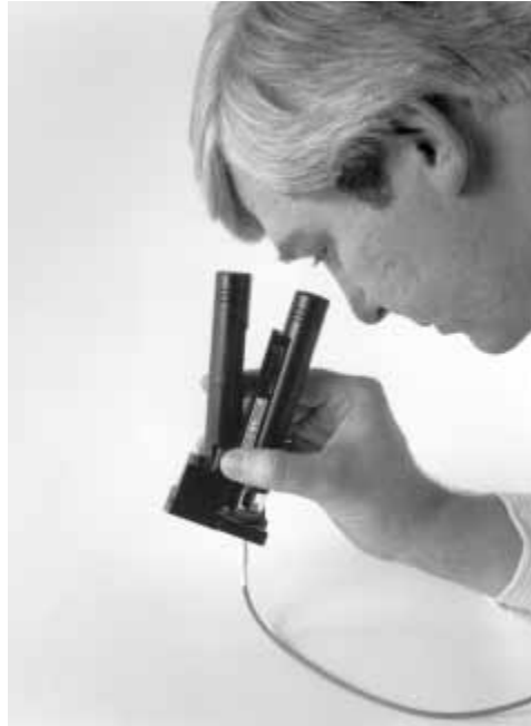
Figure 17-6 Microscopes allow inspection of connectors for polish quality, cleanliness, and faults. Courtesy Fotec, Inc.
