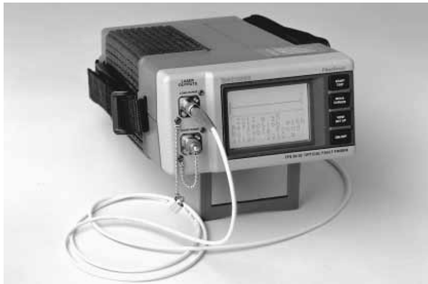
Figure 17-4c Fault finders are single OTDRs for troubleshooting. Courtesy Tektronix
